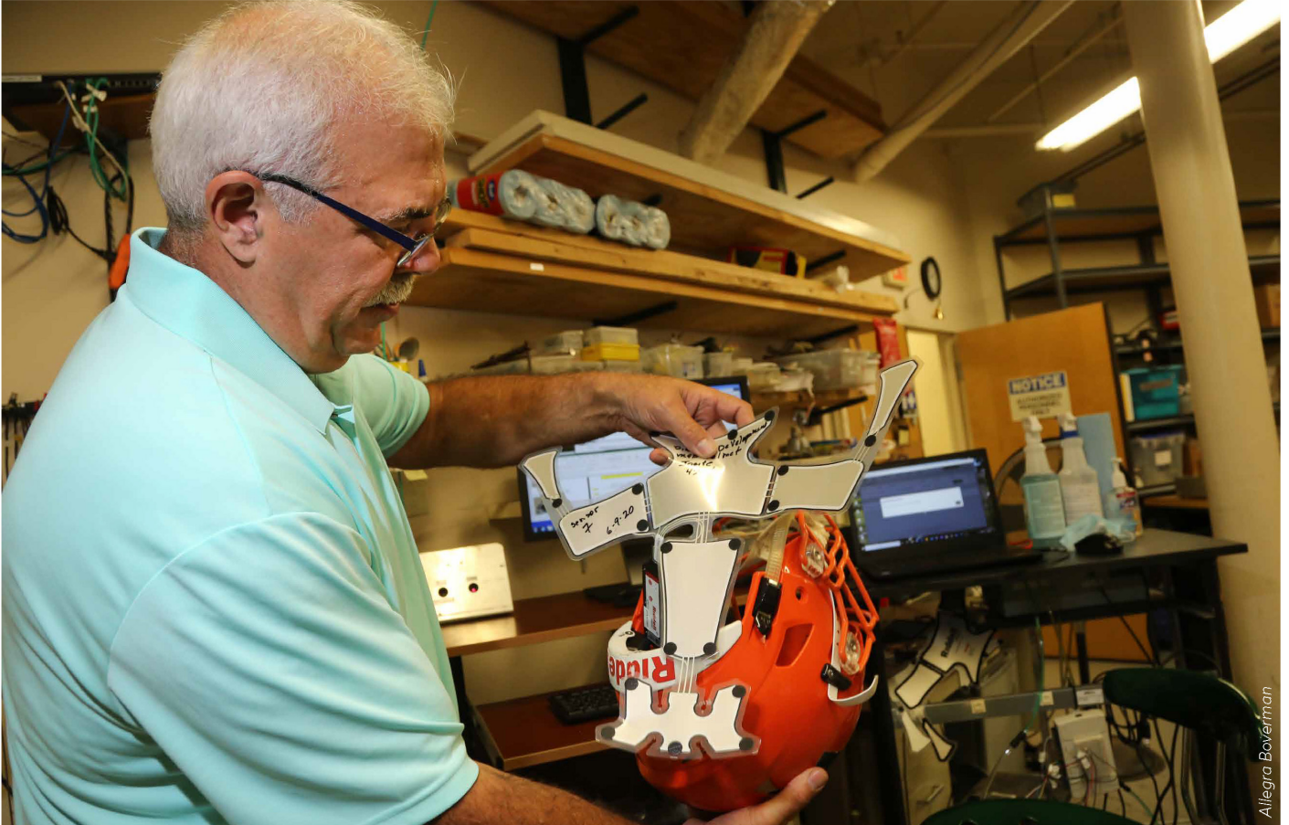
■ Mark Lefebvre, an engineering technician, of Randolph, Vermont, in the company's helmet test lab. He is showing a wearable piece that goes inside a football helmet and measures what happens to players who are playing football to help improve helmet design and help protect players.
