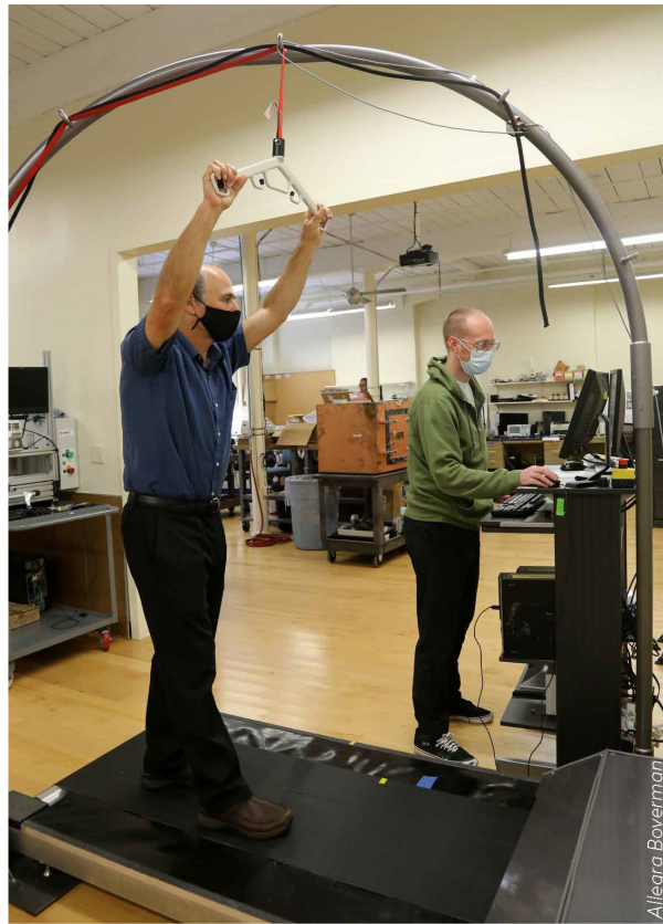
■ At Simbex in Lebanon, Rick Greenwald, the founder, and Jason Seitz, of Newport, demonstrate Active Step, a treadmill designed at Simbex for use in rehabilitation centers to help people train their reflexes to avoid falling as they age.
